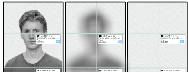
Figure 5. The dBoard in its normal mode (left), with blurred video (middle), and with privacy enabled (right).
