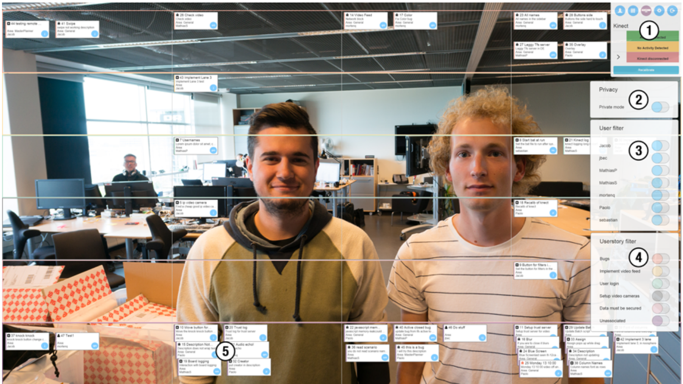
Figure 2. The user interface of the dBoard with menu (1), privacy menu (2), user filters (3), story filters (4), and tasks (5)
