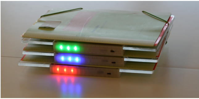
Figure 4. The color of the HyPR device can be configured to signal a wide range of things. For example, the colors can represent a specific nurse, patient status, or simply be used to highlight a patient record in an information dense environment.
