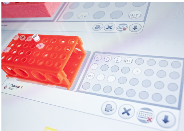
Figure 6: The eLabBench test tube rack tracking mechanism is a new kind of tabletop object integration.
