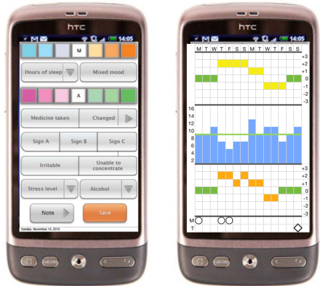
Figure 2. The MONARCA application on an Android phone. Left: The self-assessment form. Right: A graph showing data collected over two weeks on mood, sleep, activity, and medication.
