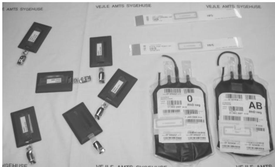
Figure 7 RFID tags (left: Wavetrend, right: ICode)
