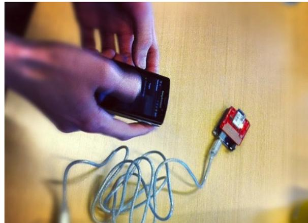
**Figure 3.** The ‘Smart Home Infrastructure’ project, where embedded controllers for the home can be easily discovered and configured for a wireless home network using an Android smart phone app.
