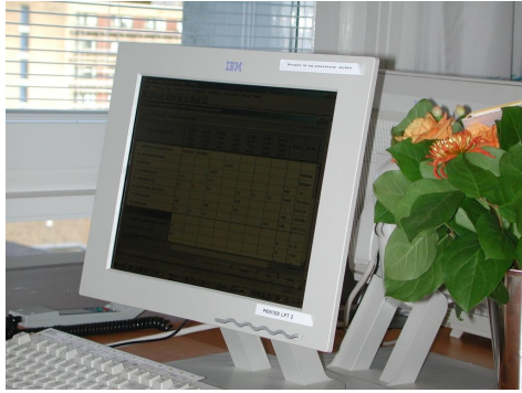
Figure 1: A terminal left on a hospital ward. Note that the user id and password are written on the top right and that the terminal has been left logged into a medical record.
