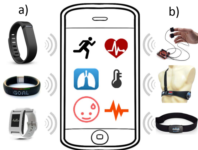
Fig. 7: Different types of sensors in external wearable devices: a) physical sensors are used for tracking of physical activity; b) bio-physiological sensors measure biological activity of the human body such as galvanic skin response, respiration or heart rate.
