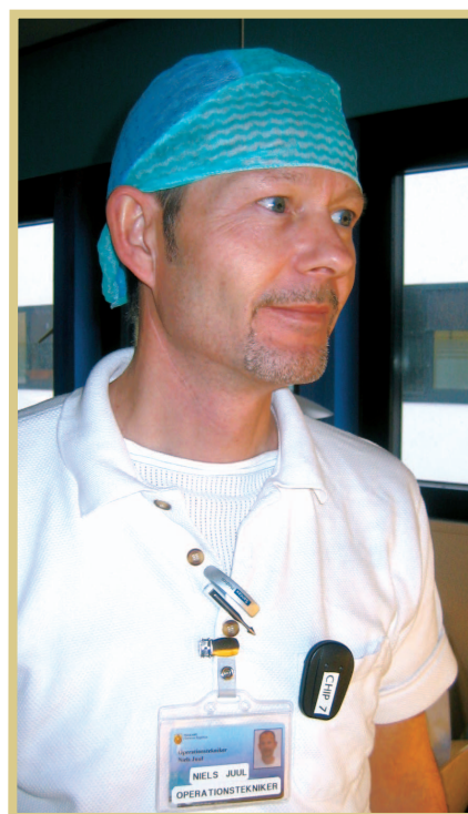
Figure 3. Tracking with Bluetooth beacons. The small black item sends a Bluetooth signal to the infrastructure. The chips are carried on the shirt or in the pocket during a work shift and then placed in a charger for the night.
