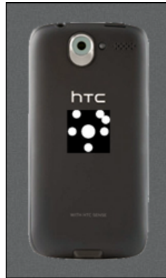
Figure 3.10: A MSS tag stuck on the back of an HTC Desire.
