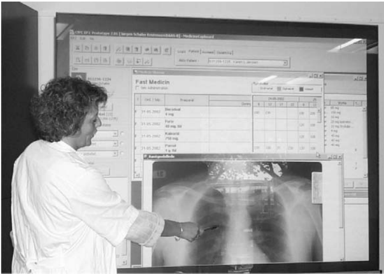
Fig. 1. A physician is using a wall-based display in a conference situation. In her hand she is holding a Personal Pen , which is used to authenticate her to the computer. An active badge woven into her white coat (not visible) is revealing her location to a context-awareness system.
