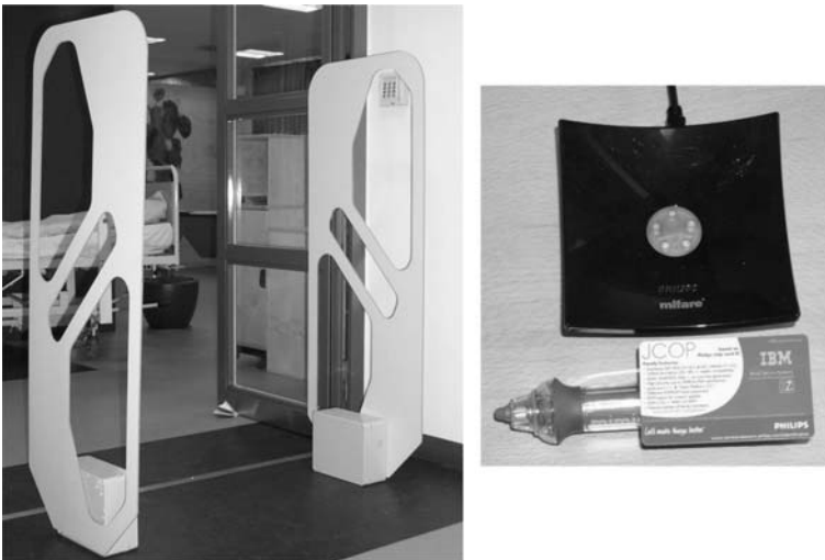
Fig. 5. Left – The ScanGate RFID Long Range Portal Antennas from Datatronic. Right – The dual-interface OpenPlatform JCOP JavaCard designed by IBM using the Philips Semiconductors' MIFARE PRO contactless reader. The JavaCard is glued to a Mimio pen, which is used at the wall-display in figure 1.
