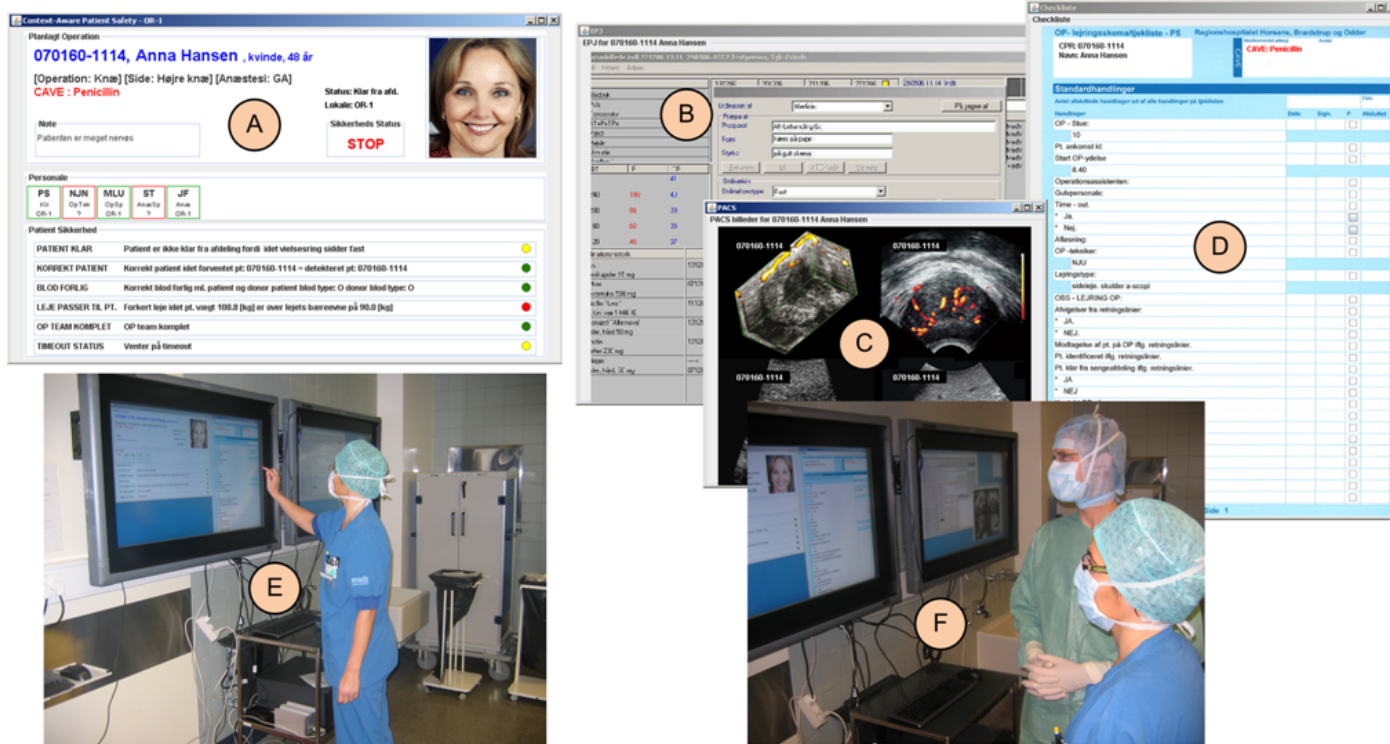
Figure 1. The CAPSIS user-interface and use. A: patient safety window, B: medical record, C: medical images, D: checklist, E: interaction, and F: reading safety status.
