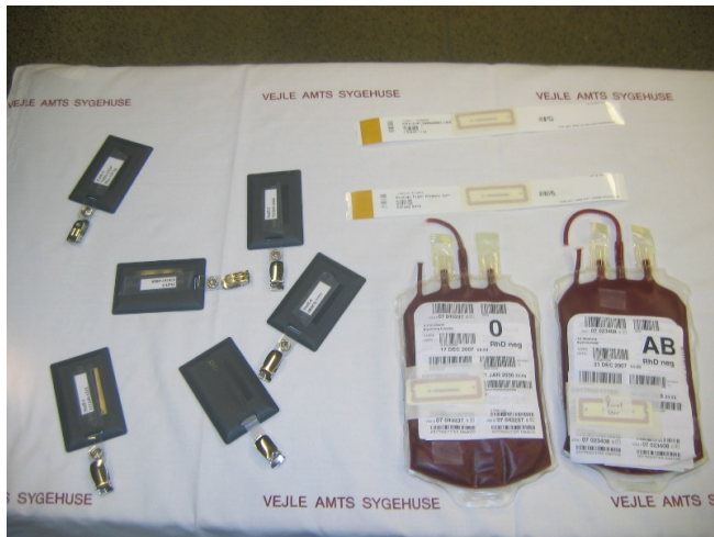
Figure 4. The RFID tags used: Passive tags are part of the patient armband used for patient identification (top), as well as for identification of blood bags (right). Active tags are used to track personnel wearing badges (left) and to tag the operation table (not shown).
