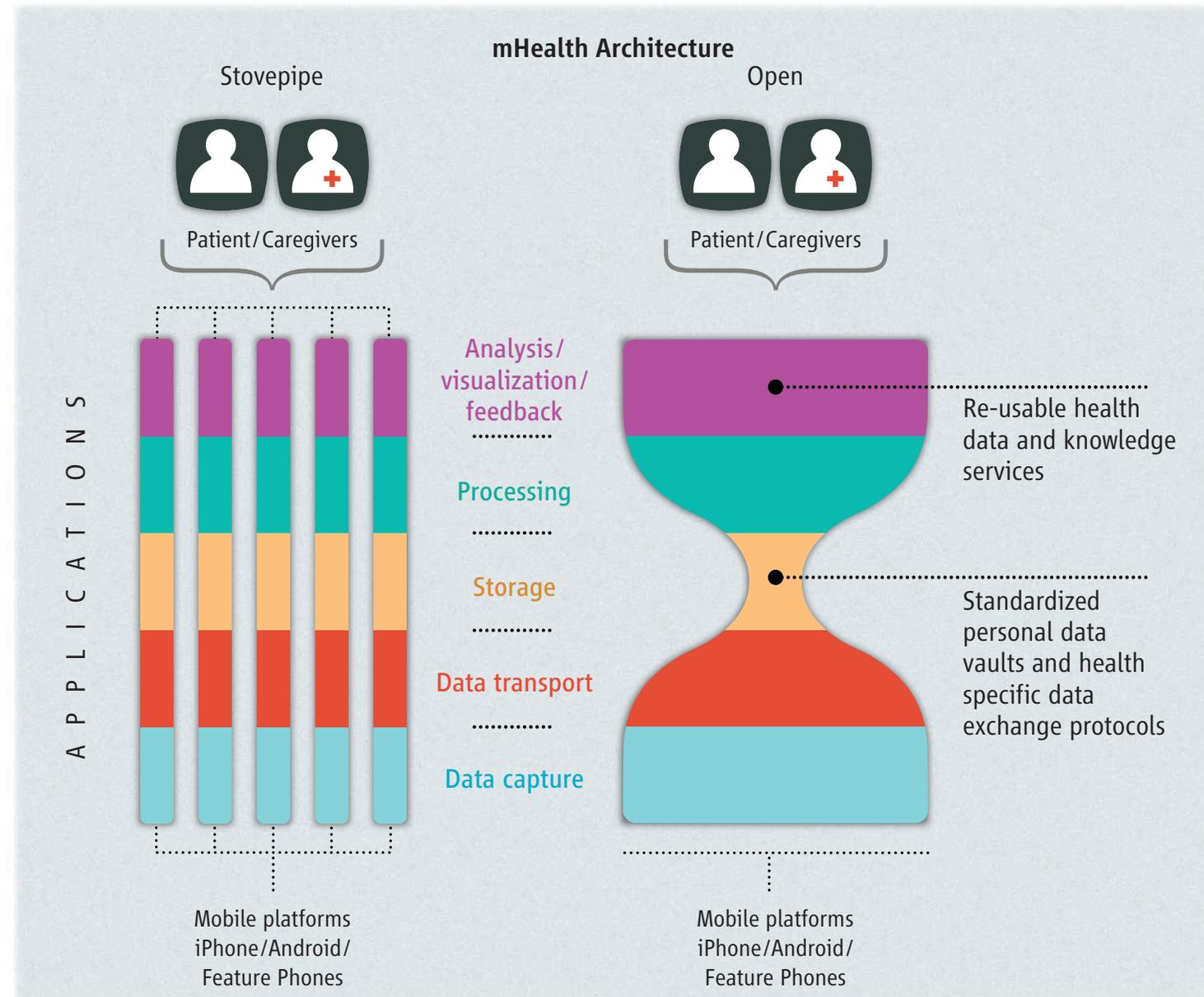
**mHealth architecture: Stovepipe versus Open.** The narrow waist of the open hourglass will include at least health-specific syntactic and semantic data standards; patient identity standards; core data processing functions such as feature extraction and analytics; and data stores that allow for selective, patient-controlled sharing. Standards should be common with broader health IT standards whenever possible.
